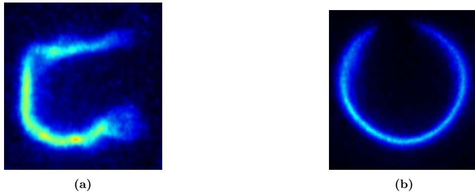
Figure 1: Chemiluminescence image obtained for non-premixed tubular flame inside the high-pressure duct. The flame is not circular due to decentralization of the inner nozzle and the breaking down of the weld while installing (left). Circular flame image of a non-premixed tubular flame is obtained outside the high pressure duct at 1 bar before damage (right)
