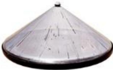
Water molecules evaporate from the salt water and leave the salt behind. The water vapor continues to evaporate and contacts the inside of the cone where it condenses and drips down and collects in a ring as fresh water.
